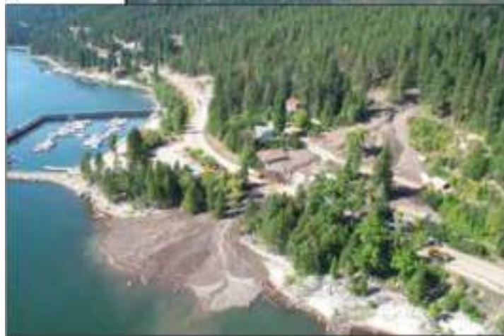
Figure 2.7. Wildfire (2003) in Kuskanook Creek headwaters with hydrophobic soils (upper). Subsequent debris flow into Kootenay Lake (lower). Photos by P. Jordan.
