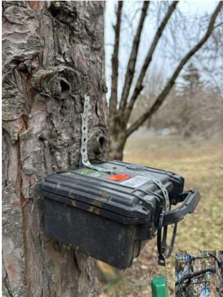
Figure 7. An acoustic Roostlogger (left) and a HOBO temperature/Rh logger installed in a chainsaw modified wildlife tree (below). Photos by Heather Gates.
