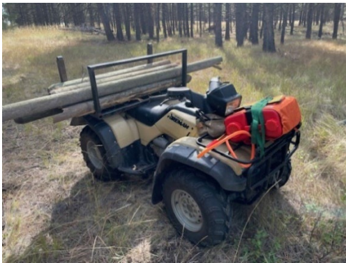
Photo 20: Note the water pack on the quad, ready for fire suppression – if needed
